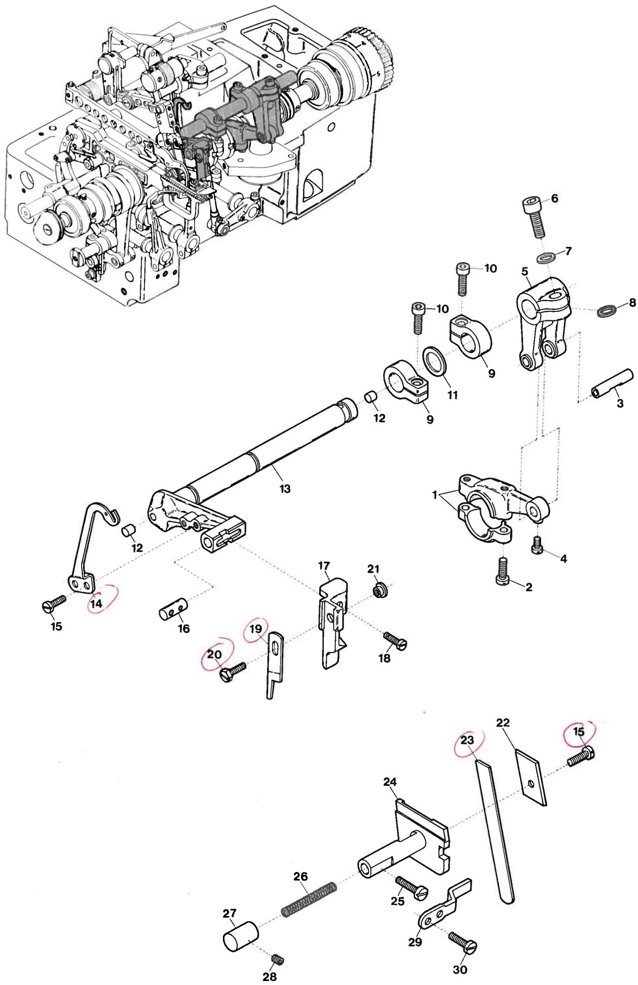
UPPER KNIFE DRIVING & LOWER KNIFE MECHANISM
