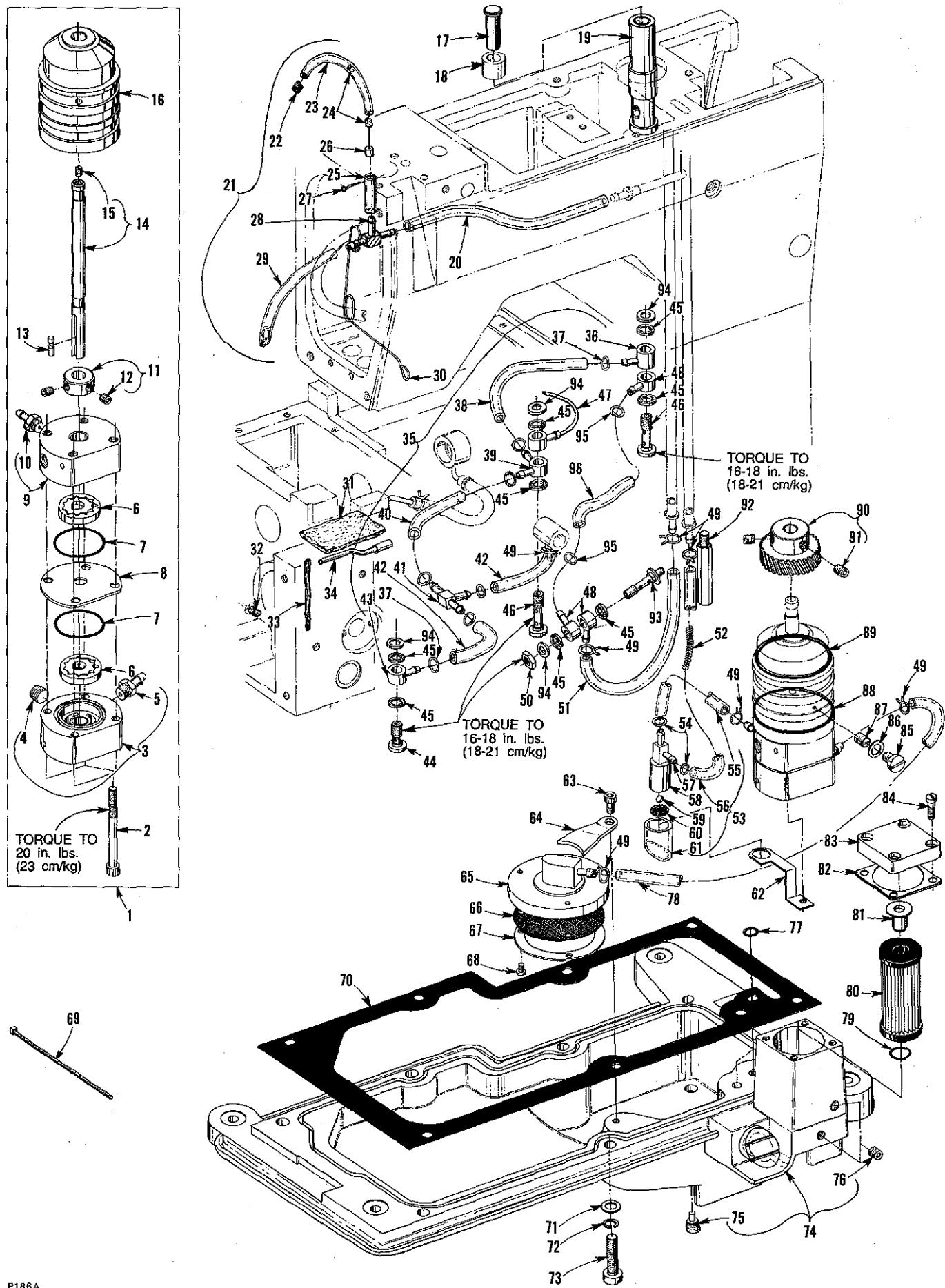
**OIL PUMP, PAN AND LUBRICATION PARTS**
