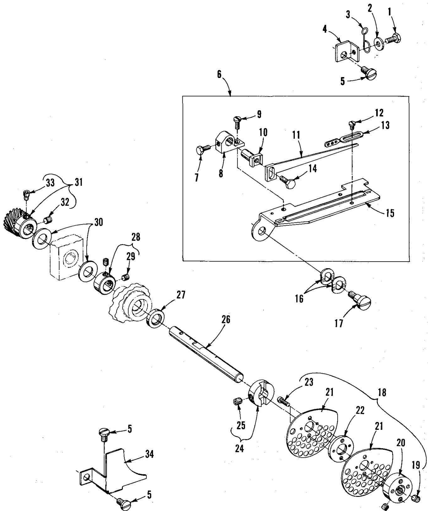
**LOOPER THREAD CAST-OFF AND DRIVING PARTS**
