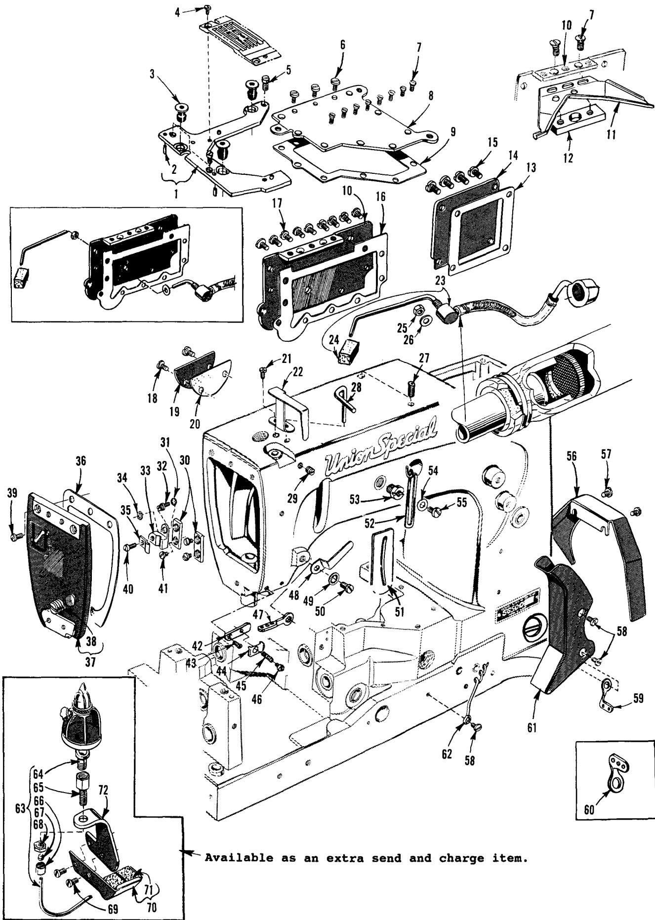
**MAIN FRAME, THROAT PLATE SUPPORT, MISC. COVERS & OILING PARTS (CONT.)**
