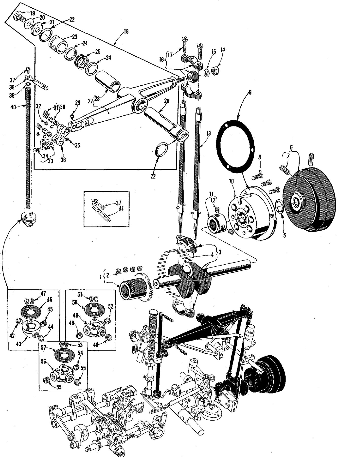
CRANKSHAFT, NEEDLE LEVER, NEEDLE BAR AND NEEDLE HEADS
