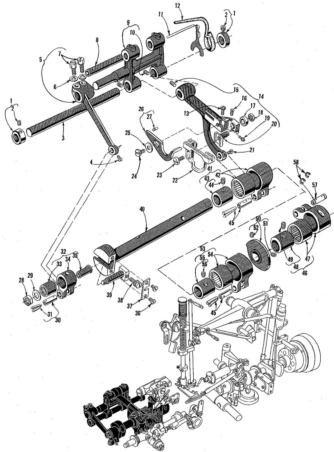
MAIN SHAFT AND FEED MECHANISM
