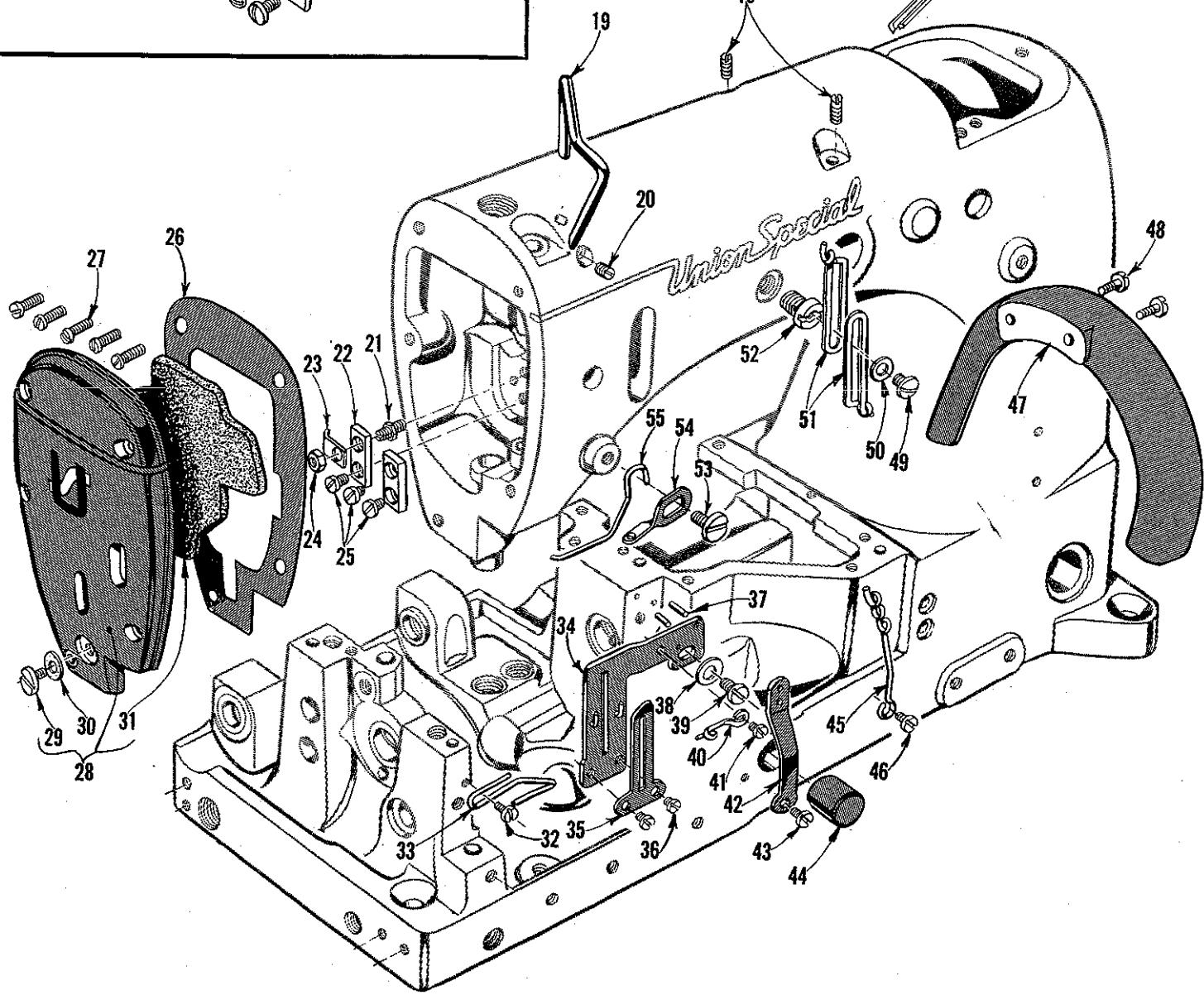
MAIN FRAME, CAST-OFF PLATE AND MISCELLANEOUS COVERS
