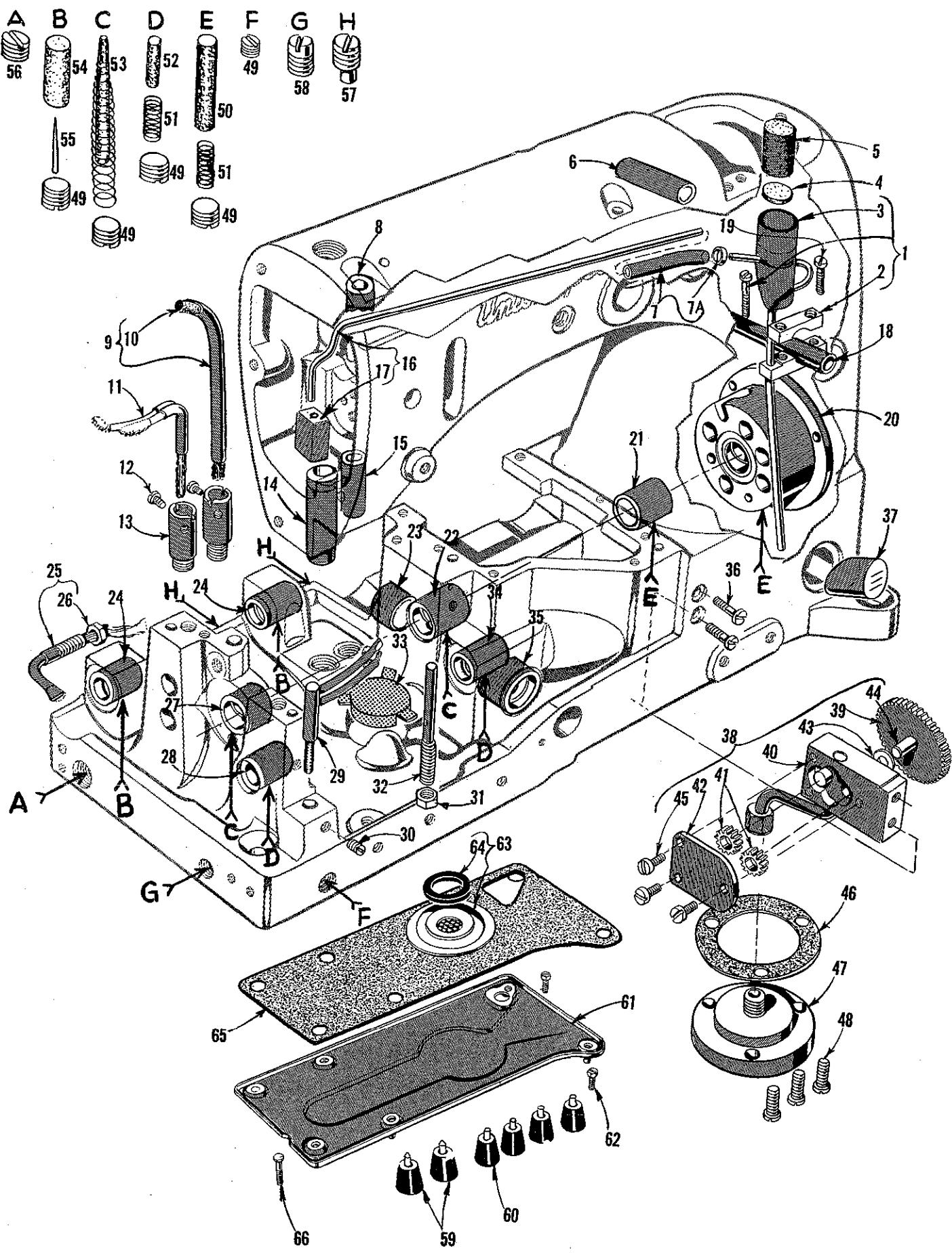
MAIN FRAME, BUSHINGS AND MISCELLANEOUS OILING PARTS
