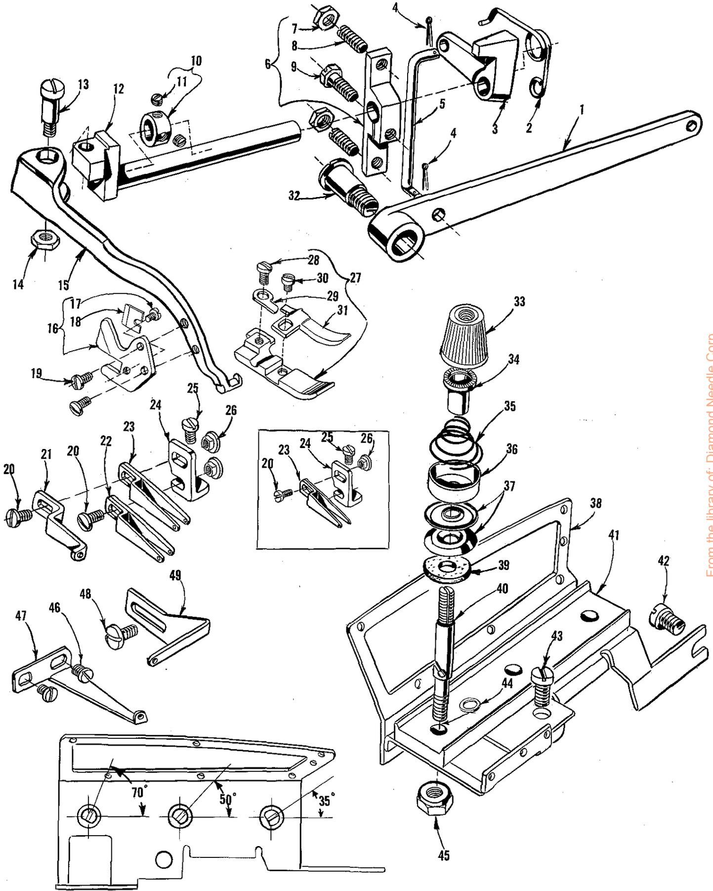
PRESSER FOOT, FOOT LIFTER, THREAD TENSION PARTS
