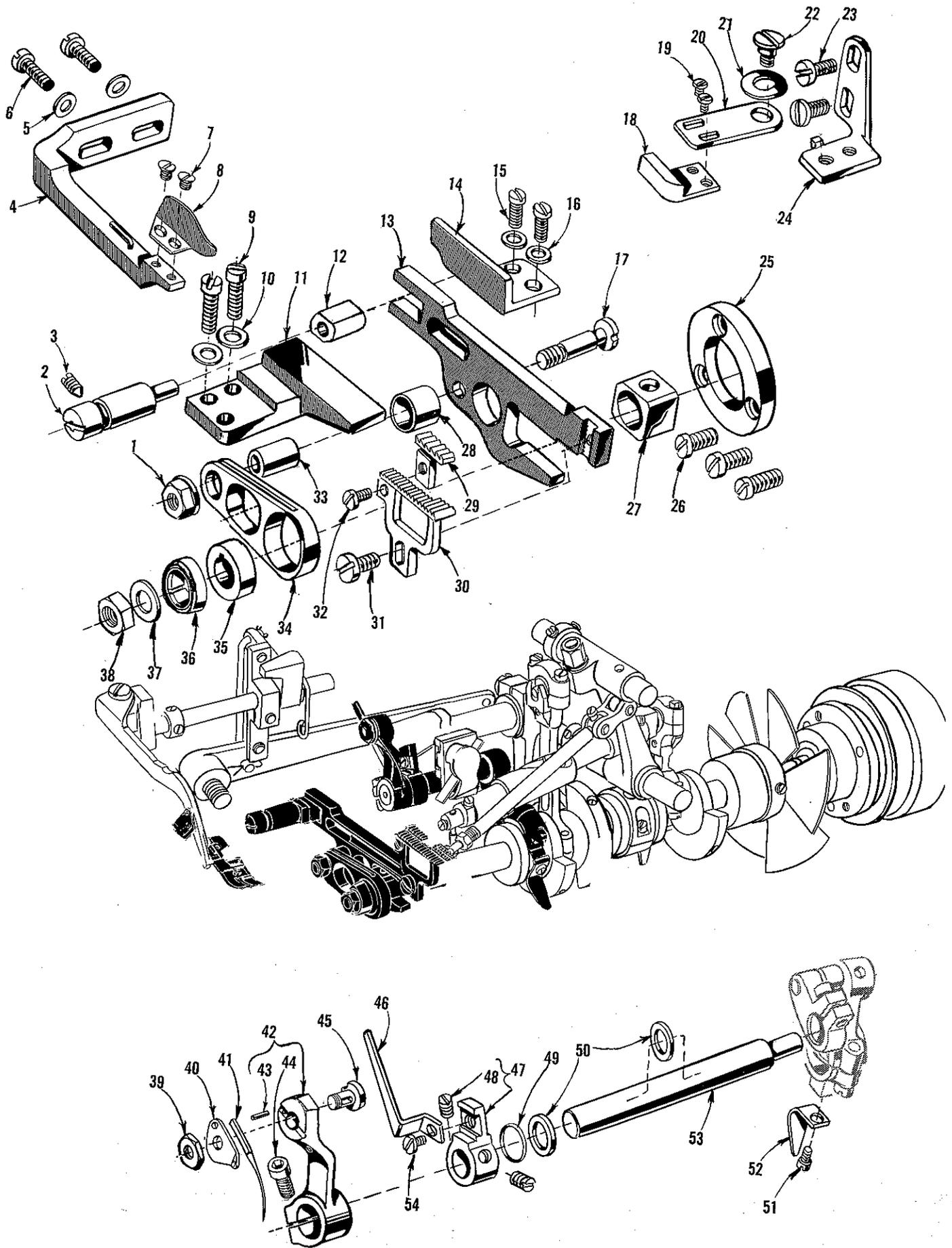
NEEDLE DRIVE AND FEED MECHANISM
