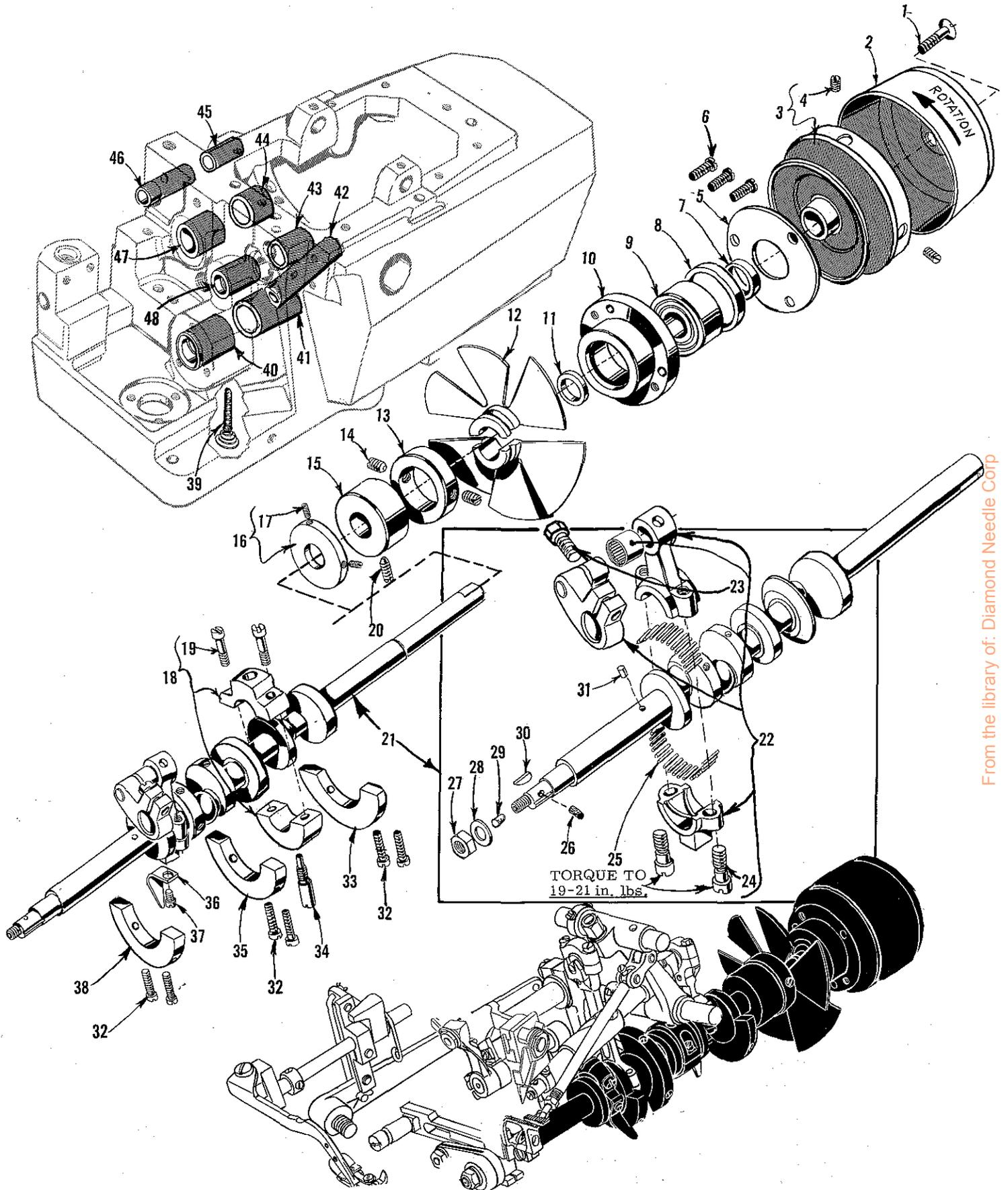
CRANKSHAFT MECHANISM AND BUSHINGS
