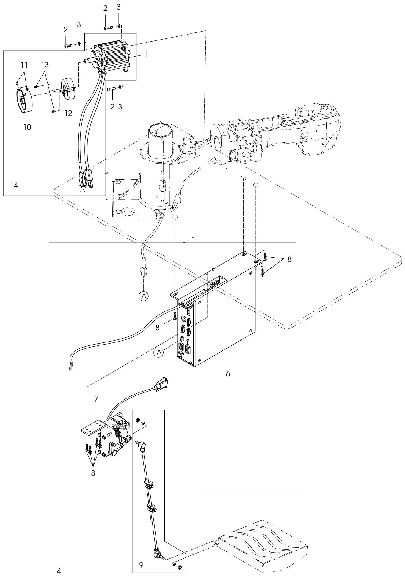
DEIRCTLY DRIVING TYPE MINI-SERVO MOTOR C.SET
