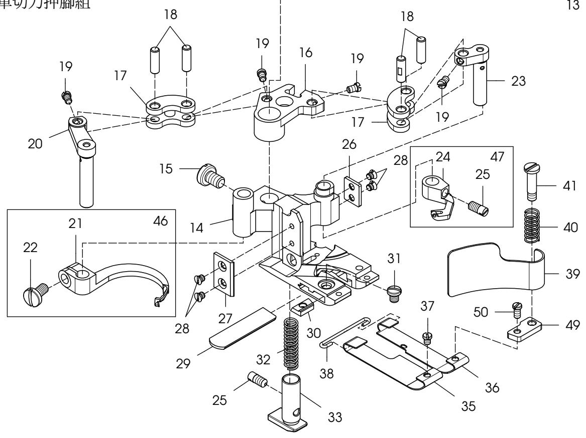
ONE SIDE CUT PRESSER FOOT MECHANISM
