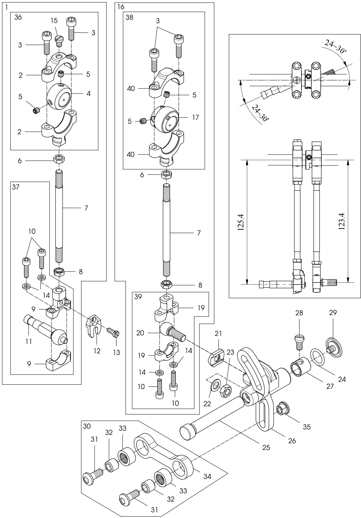
FEED DRIVING CONTROL MECHANISM
