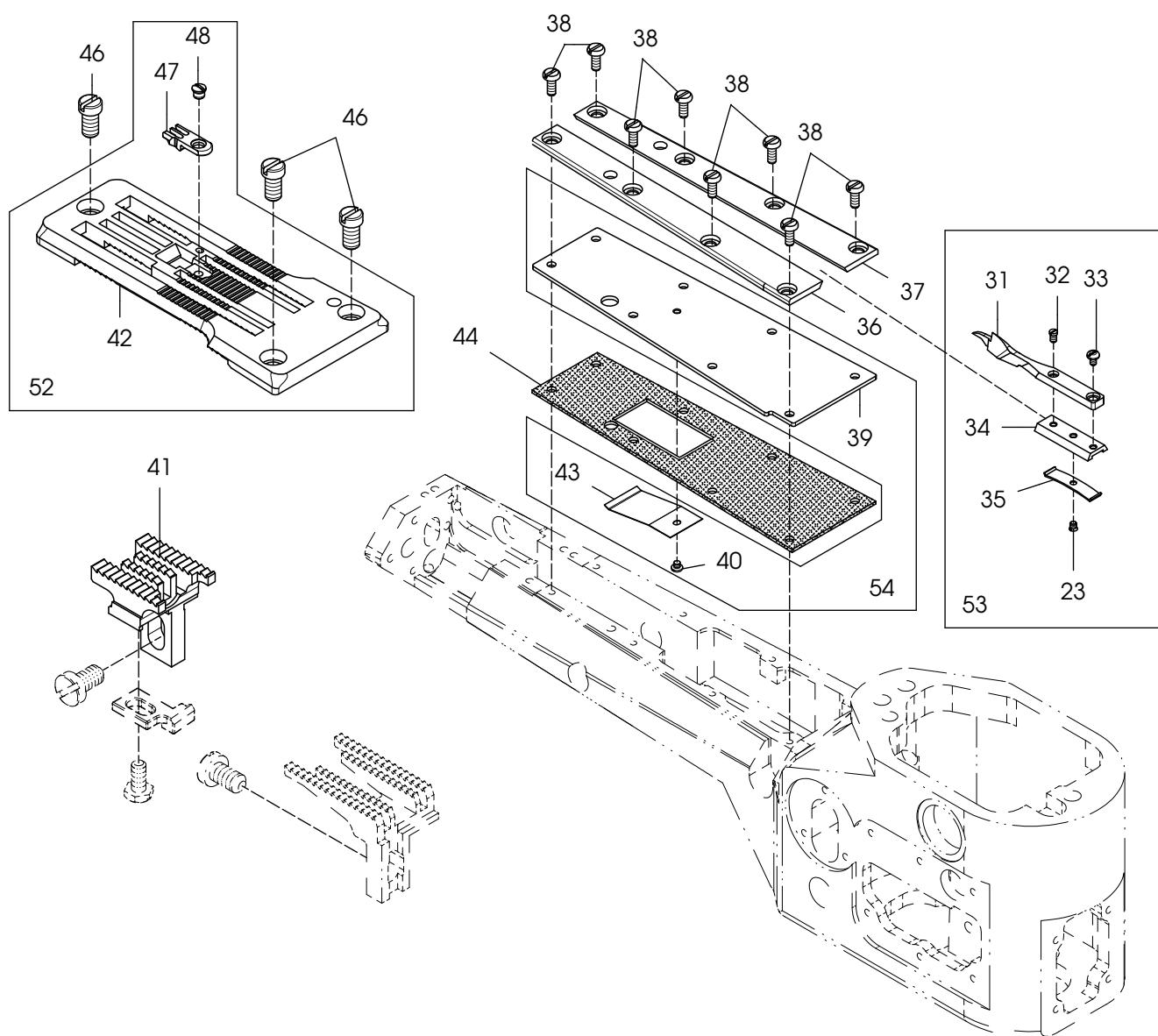
**DOUBLE SIDE CUT PRESSER FOOT MECHANISM**
