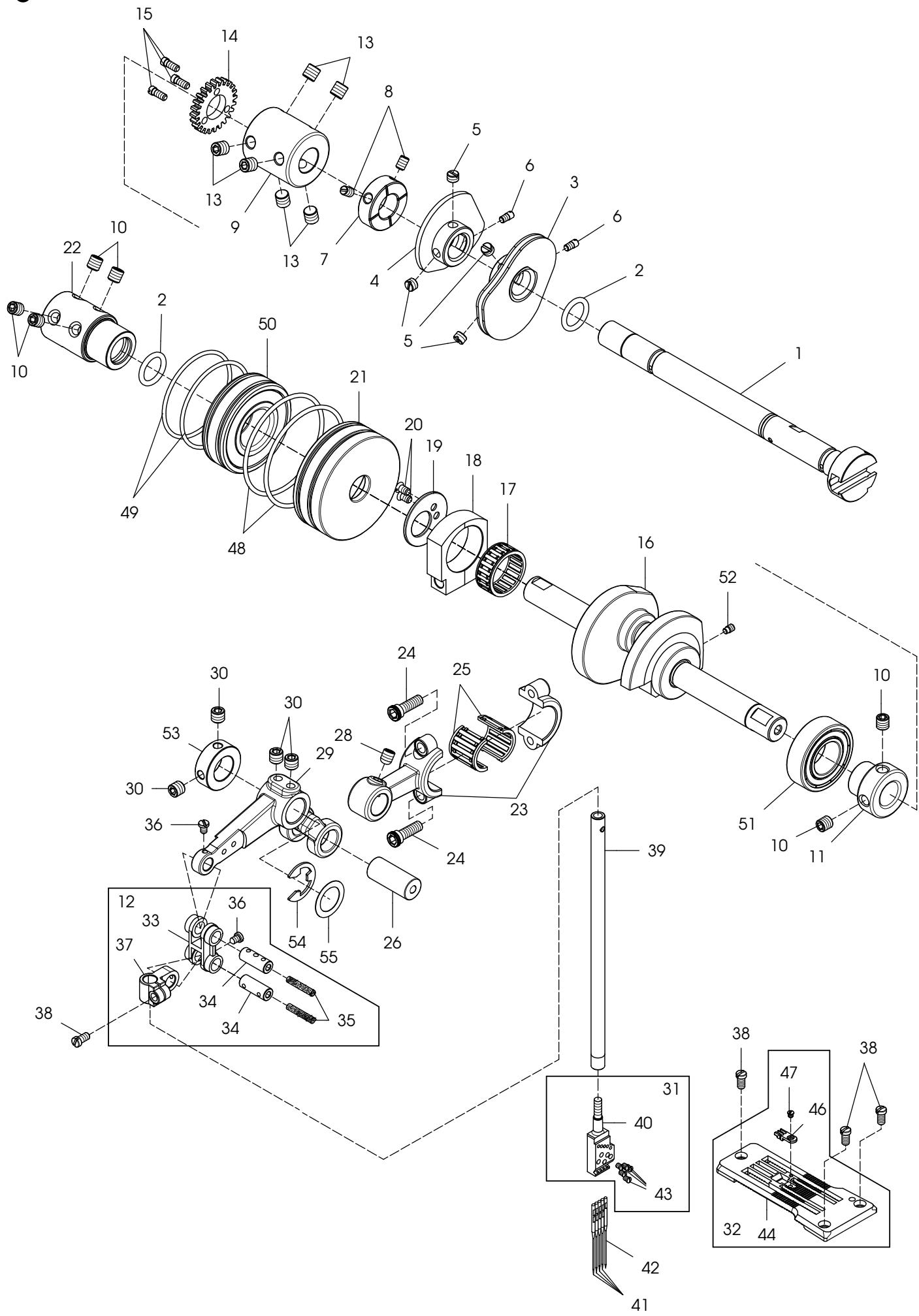
MAIN SHAFT DRIVING MECHANISM
