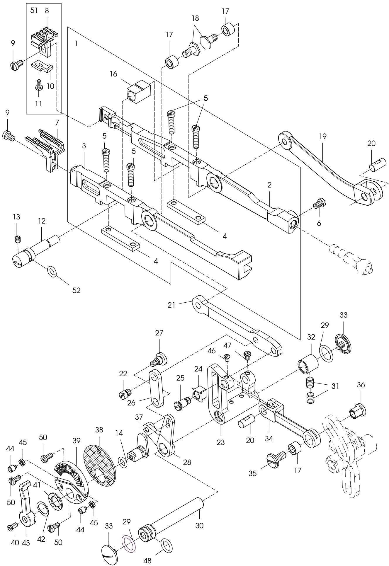
FEED DRIVING MECHANISM
