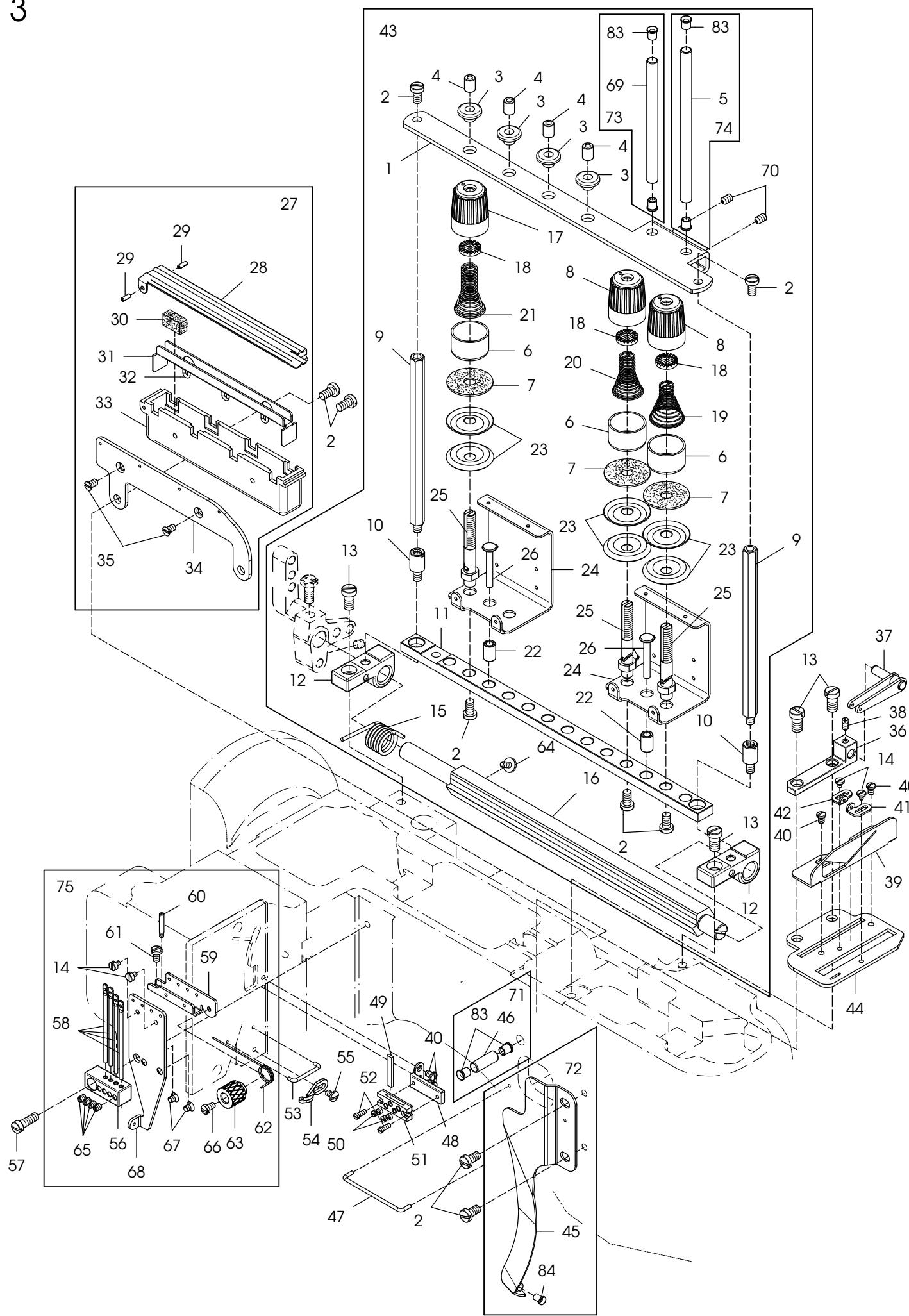
MISCELLANEOUS THREAD EYELETS-4NEEDLE
