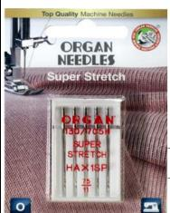
Ball point needles with special eye for highly elastic materials. Ball point alleviates making holes and scarf avoids skipped stitches.
