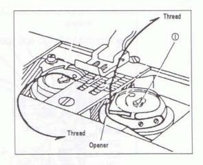
b) While holding the two needle threads by left hand, rotate the hand-wheel one turn by right hand.
