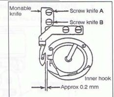
and the inner hook stopper to about 0.5 mm (the screws A and B should be loosened for this adjustment).
