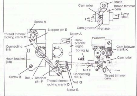
C and D to the stopper pins E and F and tighten the connecting link clamp bolt J.
