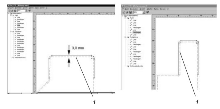
After the sewing programme has been set up by means of the Dacs739 software, contour 1 of the material clamp can be stitched to provide a template.
