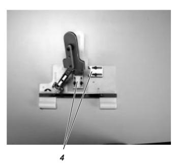
Secure material stops 4 with hexagon nuts 6 and screws 5 to the bed-plate.
