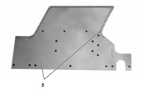
Produce edge crimp 5 of approximately 1.5 mm at the base side of the bed-plate near the seam line.
