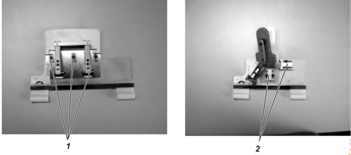
Material clamps for flaps can be equipped with up to 4 material stops 1, while clamps for waistband extensions can have max. two stops 2.
