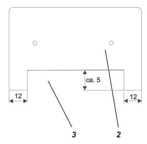
For the installation of the stops 1 on a material clamp for flaps, the clamping plate 2 has to be unlocked at the base 3.
