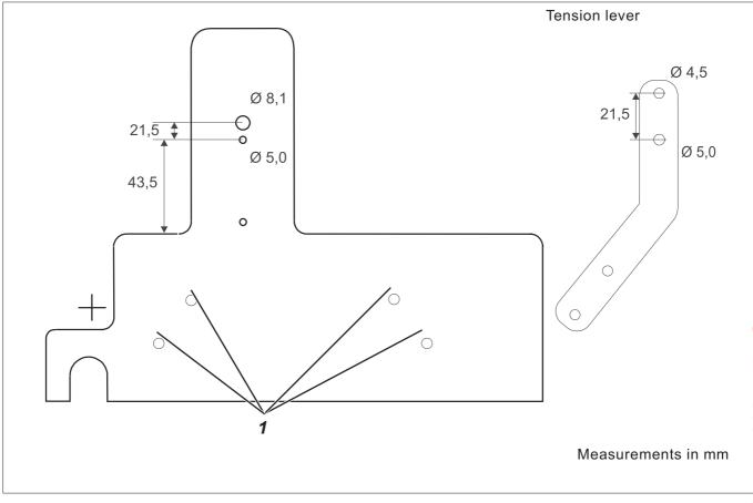
The bed-plate and the clamping plate are already equipped with holes for the clamping element. Depending on the handling, the clamping
