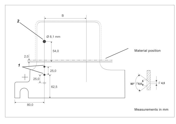
The bed-plate and the clamping plate are already equipped with holes 1 and 2 for a clamping element.
