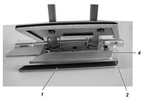
Adhere emery cloth onto the top surface of the bed-plate 1 in the area of the sewing material.
