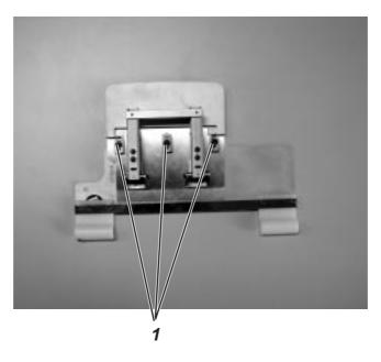
To be able to adjust the material stops 1, the intermediate sheet must be equipped with slots.
