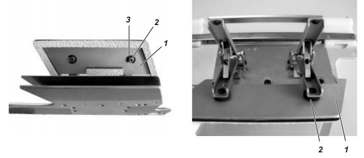
Secure clamping plate 1 with pressure piece 2 and circlip 3 at the tension levers.
