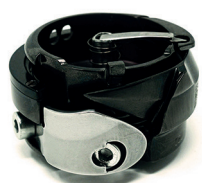
Hook 32 mm Ø Short thread trimmer
