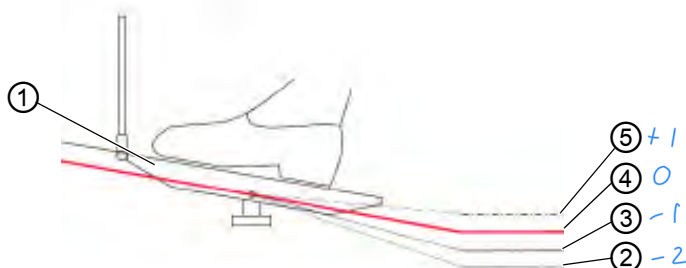
Fig. 25: Lifting the sewing feet electropneumatically
