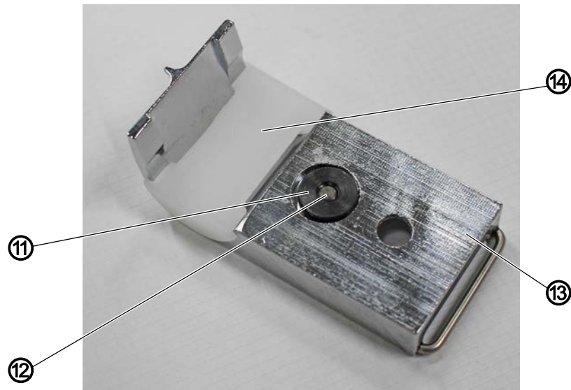
Fig. 6: Pre-assembling the guide
