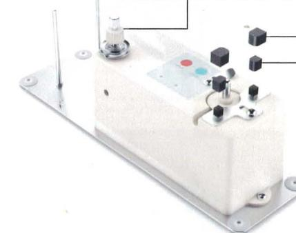
2-layer inductor cover: These 2 black inductors can be disassembled. After use, clean the dust inside the inductor to prevents the bobbin from suddenly stopping when winding. (We suggest cleaning them every 15 days)
