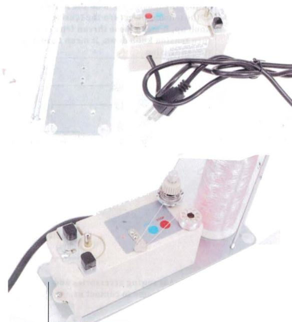
Tight the two metal screws on the bobbin winder and baseplate.
